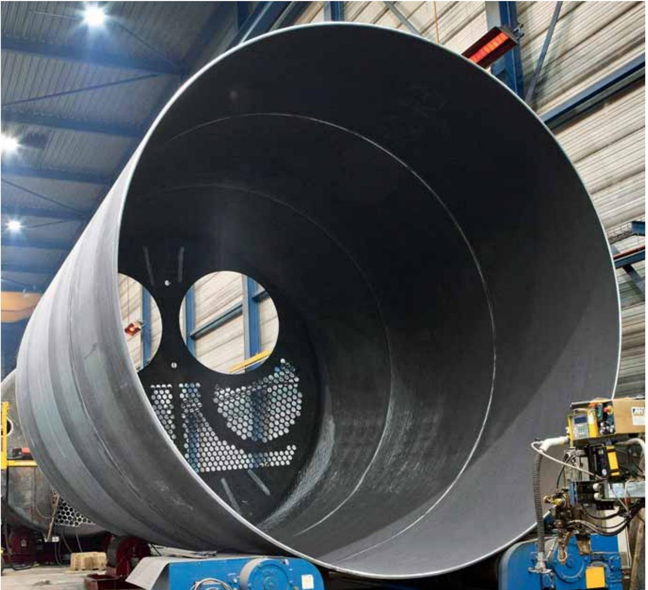
Double flame tube boilers being manufactured at HKB's facility in Venlo, Holland.
