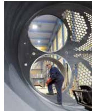
Quality inspection of a double flame tube boiler
